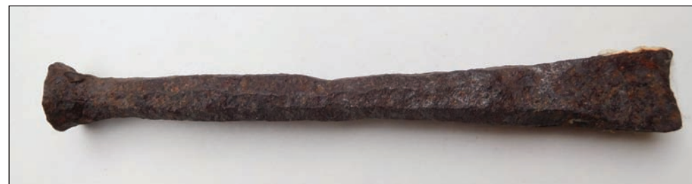
Medieval mason's chisel, as would have been used on the spire. This one was found inside stonework at the Bishop's Palace, where it had been pressed into service as a dowel.
