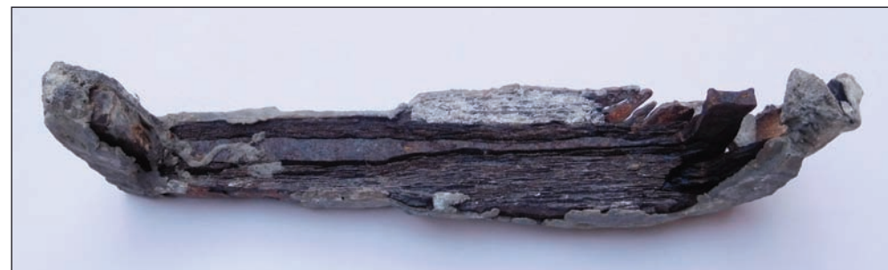
Rusted iron cramp, showing the expansion that can rip stones apart
